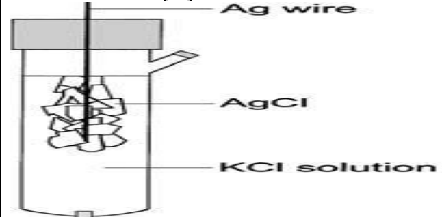
Figure 4. Typical construction of a silver/silver chloride reference electrode [19].
